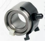
**Belgo**® Bottom roller bearings are needle roller bearings that support the bottom rollers (fluted rollers) on fine spinning machines, roving frames or drawing frames.
